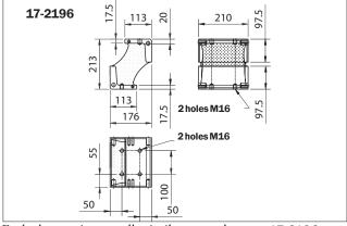
Each element is generally similar to product no. 17-2196 which may be used in pairs to provide substantially the same vertical and horizontal stiffness rates. This is similar to two sandwich mountings inclined at 45 degrees but with flat fixing surfaces resulting in simplified and compact installation.
