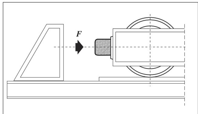
Fig. 1. Traverse crane with shock buffer ANB.
